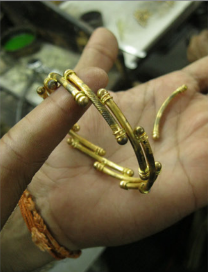
assembling of a bangle made of single elements
